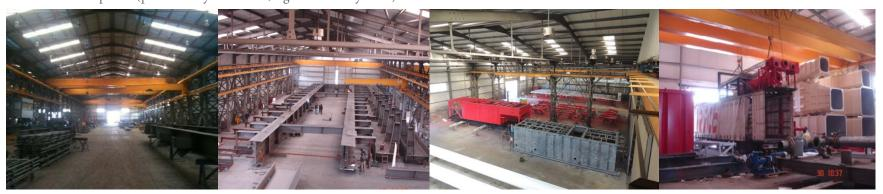
The Production Capacity is up to 1,500 tons per month in normal shift hours and the crane lift capacity per room is 100 tons.
