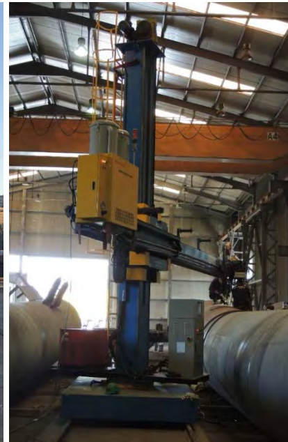
Welding boom in action performing welding operation on pipes with D1800 with 80 – 90 mm thickness for an Arch Bridge Project.
