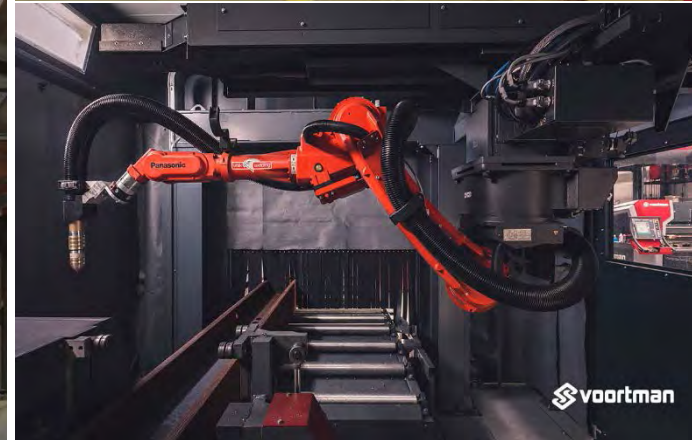
Robotic Machine V808, by Voortman, with Plasma Hypertherm 400 and Oxygen. Equipped with the new faster and more accurate versatile Panasonic TL-1800G3 coping robot.
